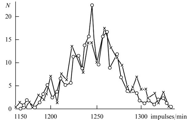
**Figure 9.** Synchronous measurements of the radioactivity of two  $^{14}\text{C}$  preparations with two independent automatic measuring stations SL-30 and SL-40 give very similar histograms. Experiment on 28 December 1980.
